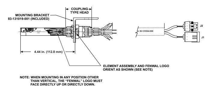
Figure 1. Diagram of KVS Detect-A-Fire
